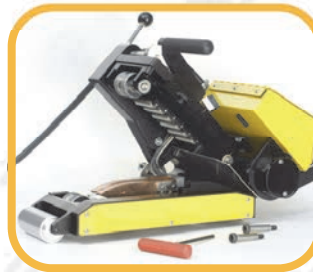
The wedge assembly can be removed in 30 seconds by simply unplugging the external heater and thermocouple plug-in wire connector, removing two shoulder bolts, and opening the frames as shown above.
